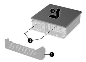
Figure 2-4 Removing the side access panel
